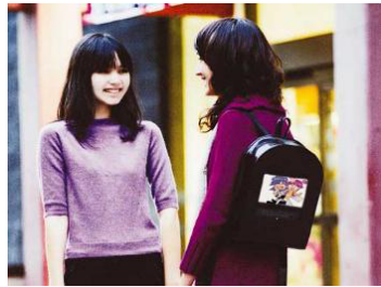
Figure 4-10: Chibi Vision is a marketing accessory which encloses a TFT monitor within a backpack.
