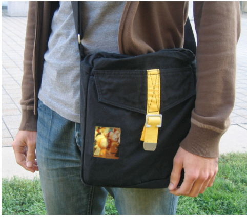
Figure 1. Urbanhermes messenger bag prototype with embedded dynamic display capabilities
