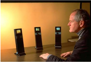
Figure 18. The Hydra four-way teleconferencing system.
