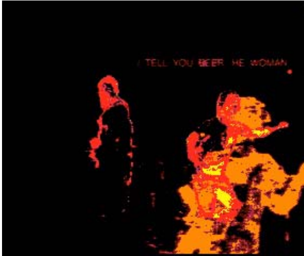
Figure 1: Current Telemurals implementation. The two images correspond to the two connected spaces. In each space, the local participants are rendered in orange, the remote participants in red.
