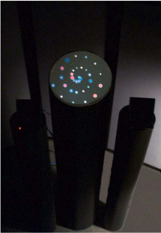
Figure 2: Large angled Visiphone display.
