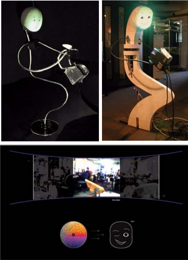
Figure 2: Top left: original avatar seat. Top right: motorized avatar seat. Bottom: remote user interface.
