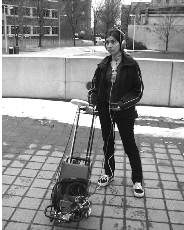
Figure 5-3: The hardware for Hear&There used in the field. The highly accurate GPS receiver is rather large, so we have attached it to a luggage cart.
