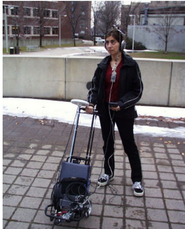
Figure 2. The navigation toolkit, including a GPS receiver, a laptop computer, headphones with an attached digital compass, and a PalmPilot. Because the high-accuracy GPS receiver is rather bulky, we have placed it on a luggage cart that the user can roll around the environment.
