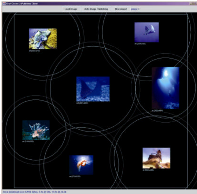
Fig 4: Picture publishing interface in Chat Circles II. As the administrator posts pictures in the chatroom, she has control over the size of the viewing range for each picture, which is represented as a circle around each image.
