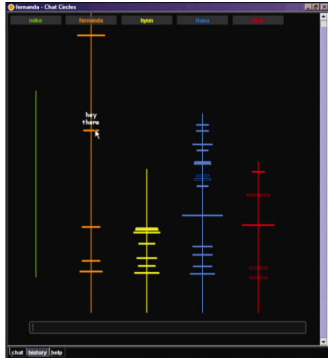
Fig 2: Chat Circles history interface. Each vertical line represents a user. The horizontal bars represent posting, with hollow bars standing for messages posted outside the local user's hearing range. The text of postings, shown as solid bars, can be retrieved by mouse-over.
