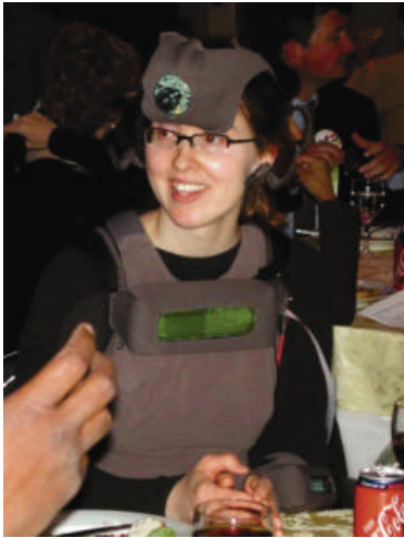
Fig. 9: TeleActor wearing gear: head-mounted camera and speakers, microphone, chest display and arm display.
